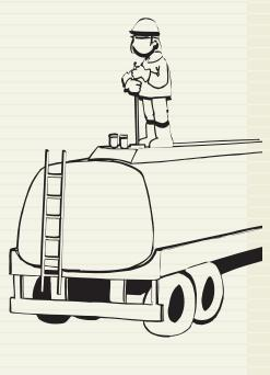
When the tank bottom sampler touches the bottom it is filled with the liquid from the bottom.
