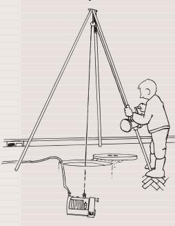
The bailer is operated with the aid of the light lifting set.
