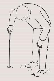
The (horizontal) measurement of the penetration resistance in the wall of a profile pit.
