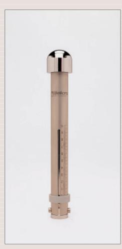
Hand penetrometer for top layers
