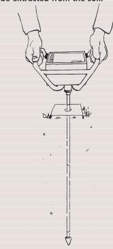
The penetrologger is fitted with touch control.
