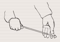
The cone check is used to inspect the wear of the cones.
