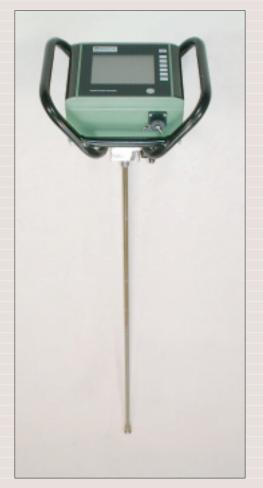
Penetrologger, probing rod and cone
