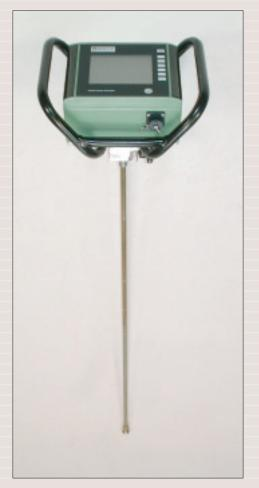
Penetrologger, probing rod and cone
