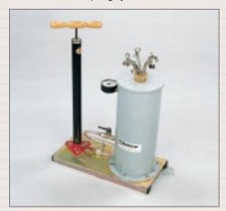
Vacuum tank with vacuum pump
