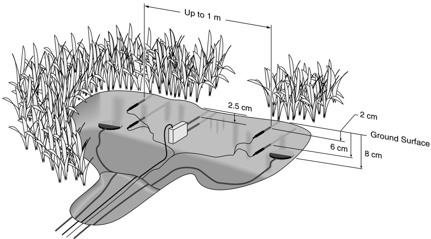
The above illustration shows heat flux sensors installed with the CS616 and TCAV Averaging Soil Temperature Probes. All sensors must be completely inserted into the soil face before the hole is backfilled.
