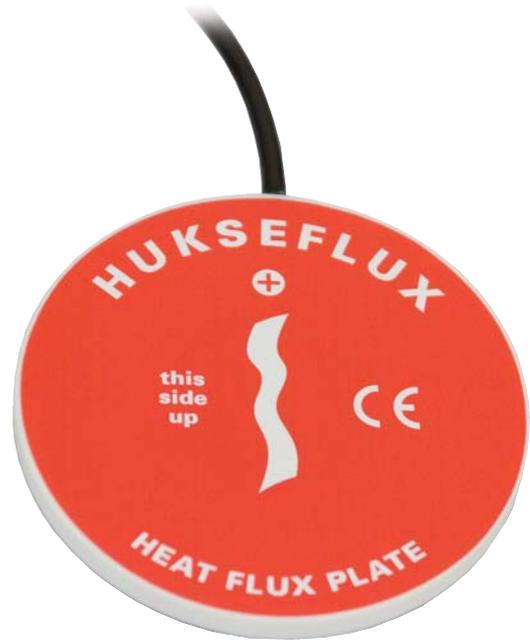
The HFP01 is for applications that do not require self calibration.
