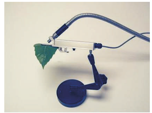
Optional - Standard PAR Clip mounted on articulating arm stand for lab work.
