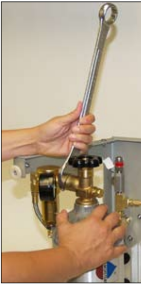
Fig. 16 - Removing the tank by loosening the bolt.
