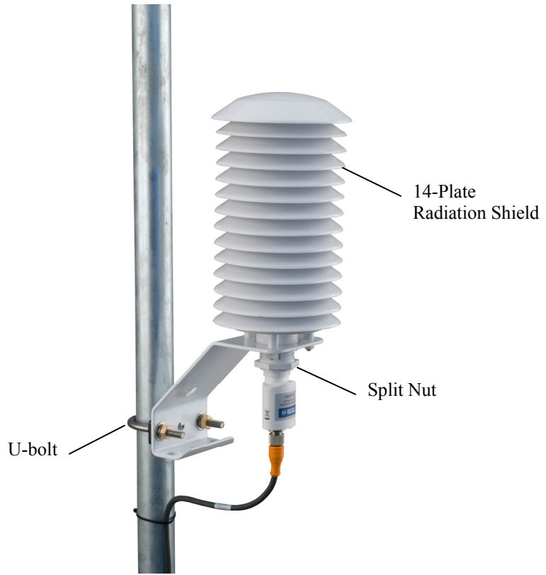
FIGURE 4-1. HMP155A and 14-plate radiation shield on a tripod mast
