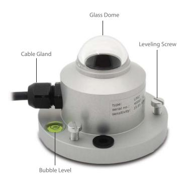
The LP02's bubble level and adjusting screws allow the pyranometer to be leveled without using a leveling base. The cable gland makes it easier for the user to change cables.
