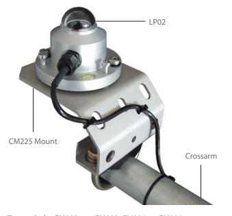
To attach the CM225 to a CM202, CM204, or CM206 crossarm, place the U-bolt in the holes on the bottom of the bracket.
