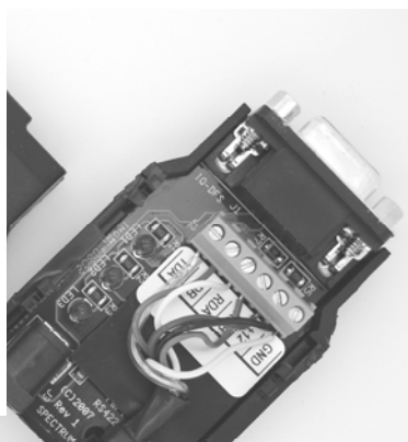
Second Generation Connector Box - Interior View (with Terminal Block)
