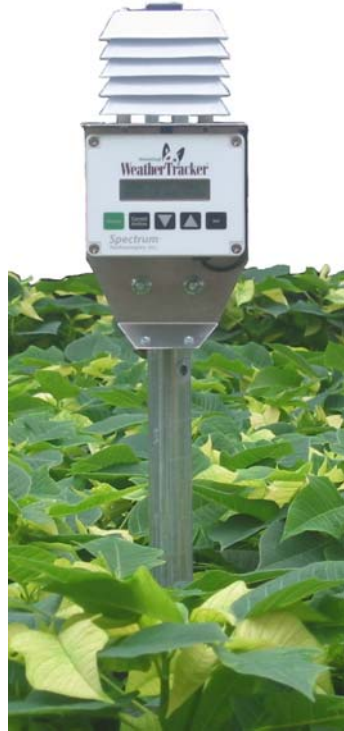
Figure 1: WeatherTracker mounted on 1" conduit
