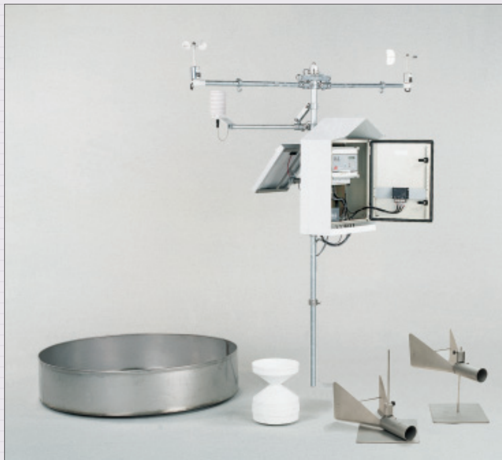
Automatic agro-meteostation, 62 channels
