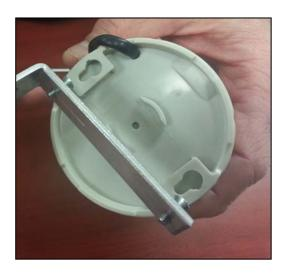
Mount the bracket, with the screw heads sliding into the small end of the slot. Turn the screws until they are hand tight.
