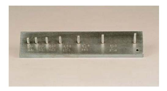
Used to measure the length of individual particles and classify aggregate elongation to BS812-105.
