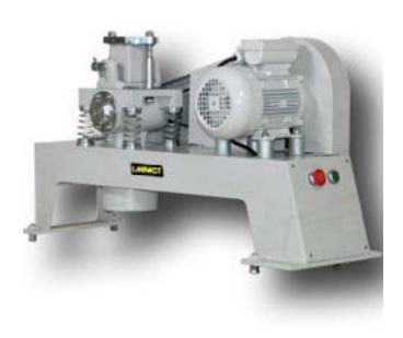
A vibrating platform with eccentric mechanism holds the mould and vibrates it at a frequency of 12,000 cycles per minute. The rigid steel frame is complete with drive cover, time switch and a starter control
