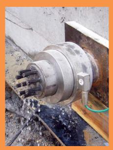
Abutment plates are normally designed to suit specific site requirements. In all cases the minimum abutment thickness should the thickness of the load distribution plate. The abutment plate surface area must be greater than the load cell area. Load distribution plate and load cell have the same central hole diameter.
