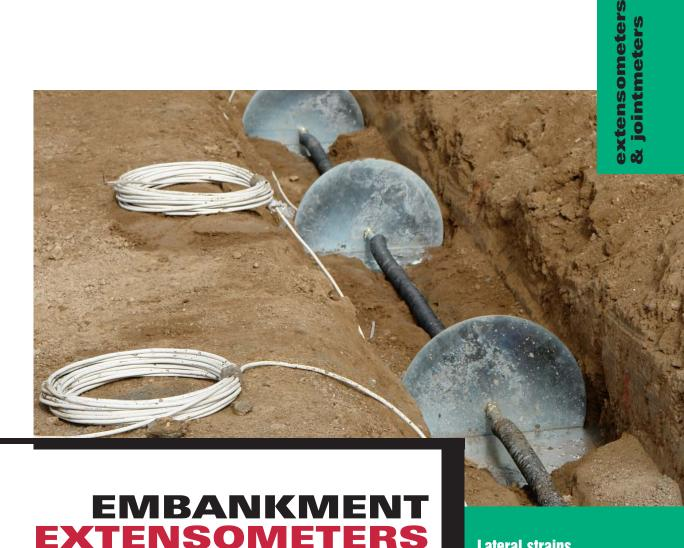
Embankment extensometers are used to measure soil strains in large earth structures.
