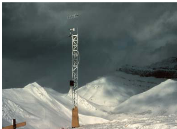
Meteorological conditions measured at Lake Louise, Alberta, Canada are telemetered via phone-to-RF link to a base station.
