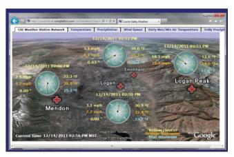
CSI Web Server was used to simultaneously display data from multiple dataloggers on one web page.
