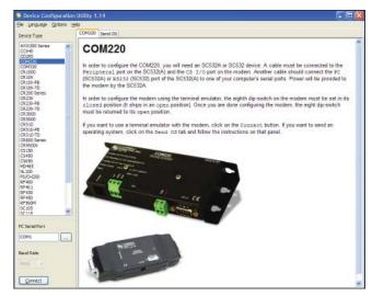
Our device configuration (DevConfig) utility is bundled with PC400, LoggerNet, and RTDAQ and can be downloaded, at no charge, from our website. DevConfig is used to change device settings and update operating systems.
