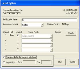
Set the measurement interval ranging from 1 to 120 minutes and ensure all channels are enabled. The Delay Start option allows you to start logging data at a later time.
