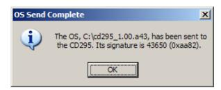
6. Once the download is complete, disconnect power from the CD295 for at least 30 seconds to ensure that it has been completely reset. After this, the new operating system will run.
