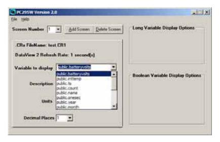
6. The 'Description' and 'Units' fields are free-form text strings that are displayed on the CD295 along with the value collected from the datalogger. These fields can be used to provide a user friendly description and engineering units of the value displayed. It is also possible to choose the number of decimal places to be used when displaying the value.
