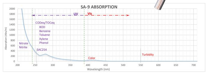
The validated spectral calibration by SA-9 uses multiple wavelengths to monitor and compensate each sum parameter,
