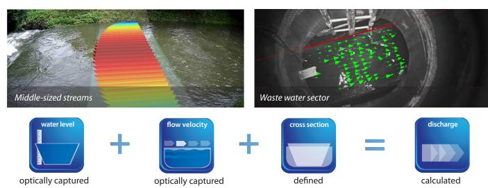
The surface velocity profile is measured optically using a patented cross correlation approach, SSIV. The water level detection is carried out simultaneously by an image processing technique. The vertical velocity profile is obtained following ISO standard EN ISO 748:2007. Integrating the velocity over the river width yields the discharge.
