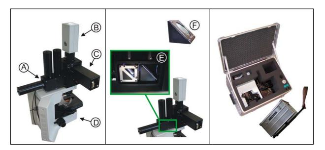
The **Micro-FluorCam** is used to characterize, on cellular and sub-cellular levels, dynamics and spatial heterogeneity in fluorescence emission of plants by Kautsky effect, quenching analysis, and other dynamic fluorescence features.
