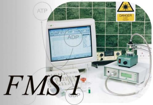
"The FMS1 is a pulse modulated chlorophyll fluorimeter with mains power supply for laboratory/near field use. It is suitable for non-invasive sampling under natural light conditions & may be interfaced with our range of oxygen electrode chambers for simultaneous oxygen measurements."
