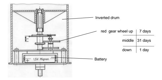
Place the recording strip onto the inverted drum (see 6.1 Changing the recording strip) and insert this onto the drive mechanism until it locks into place!
