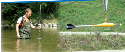
Flow measurement with universal current meter F1
