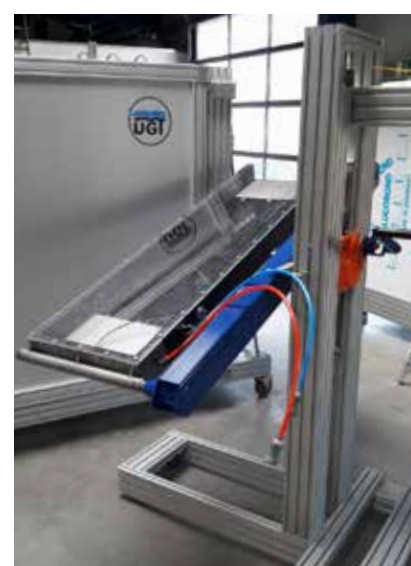
Trolley for removing and inserting the chambers
