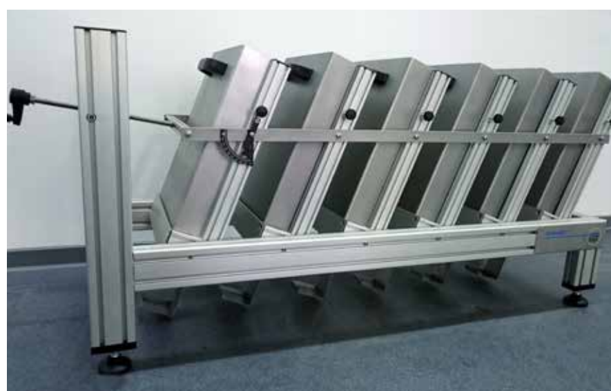
Rhizotron block for the reception of rhizotron chambers with a window size of approx. 30 x 42 cm
