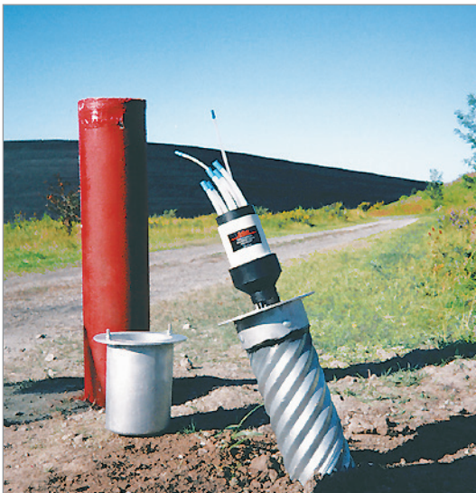
An investigation of hydraulic properties beneath a large waste site. Waterloo Multilevel Systems were chosen to allow water quality sampling and to help determine the zones of highest permeability within the aquifer.
