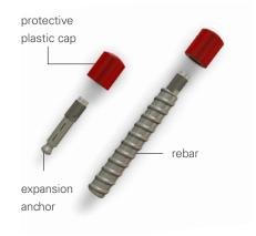
Threaded reference bolts consist of a 3/8" stainless steel head mounted on a steel rebar (Ø 22 mm) or on an expansion anchor (Ø 14 mm).
