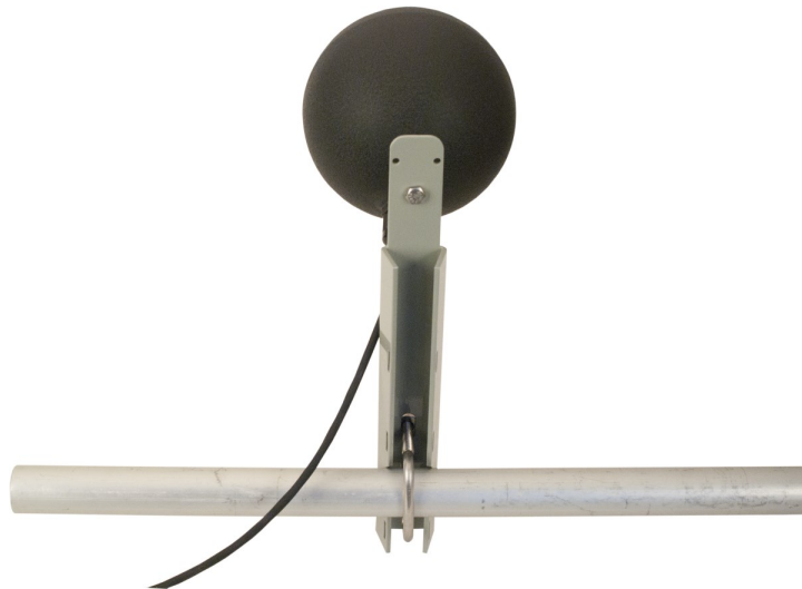
Figure 7-5. BlackGlobe mounted to a crossarm (back view)
