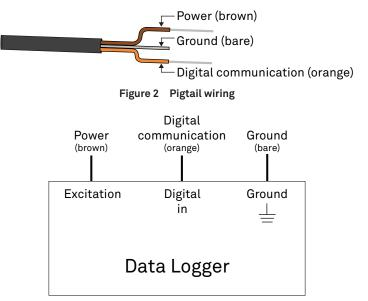
Figure 3 Wiring diagram
