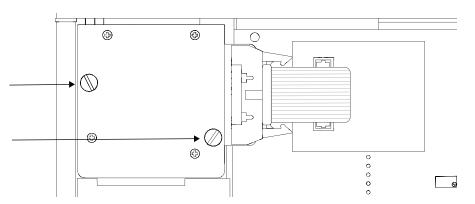
Figure 22 Thumb screws
