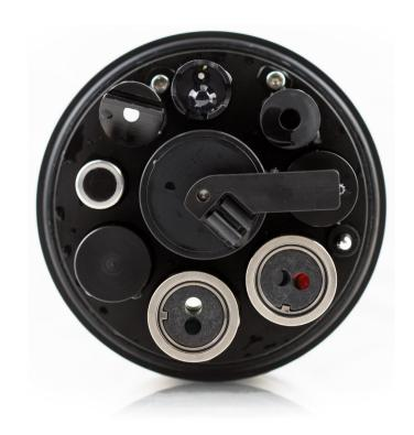
The Manta+F35 includes the same standard sensors as the +35, with the option to add up to three fluorometers. The +F35 features an antifouling copper-infused "nose cone" covering the sensor bodies. A central wiper system keeps the exposed sensor surfaces clean during continuous deployments. These features mean better data and less overall cleaning is required. PAR,  $CO_2$ , TDG, and ISE sensors are unavailable on the +F35.
