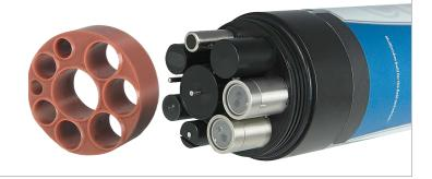
**The Manta+40** comes standard with turbidity, temperature, pH, conductivity, and dissolved oxygen sensors, with the option to add ORP and depth sensors. In addition to these standard sensors, the M+40 will accommodate three fluorometers (medium sensors) plus three ISE sensors (small sensors).
